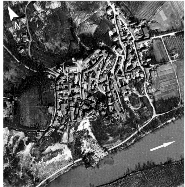
Figure 5 – Aerial photograph of the village of Montecastello. The slump-earth flow of 9 March 1978 is clearly visible on the southern slope. The displaced material partially dammed the Tanaro riverbed.
