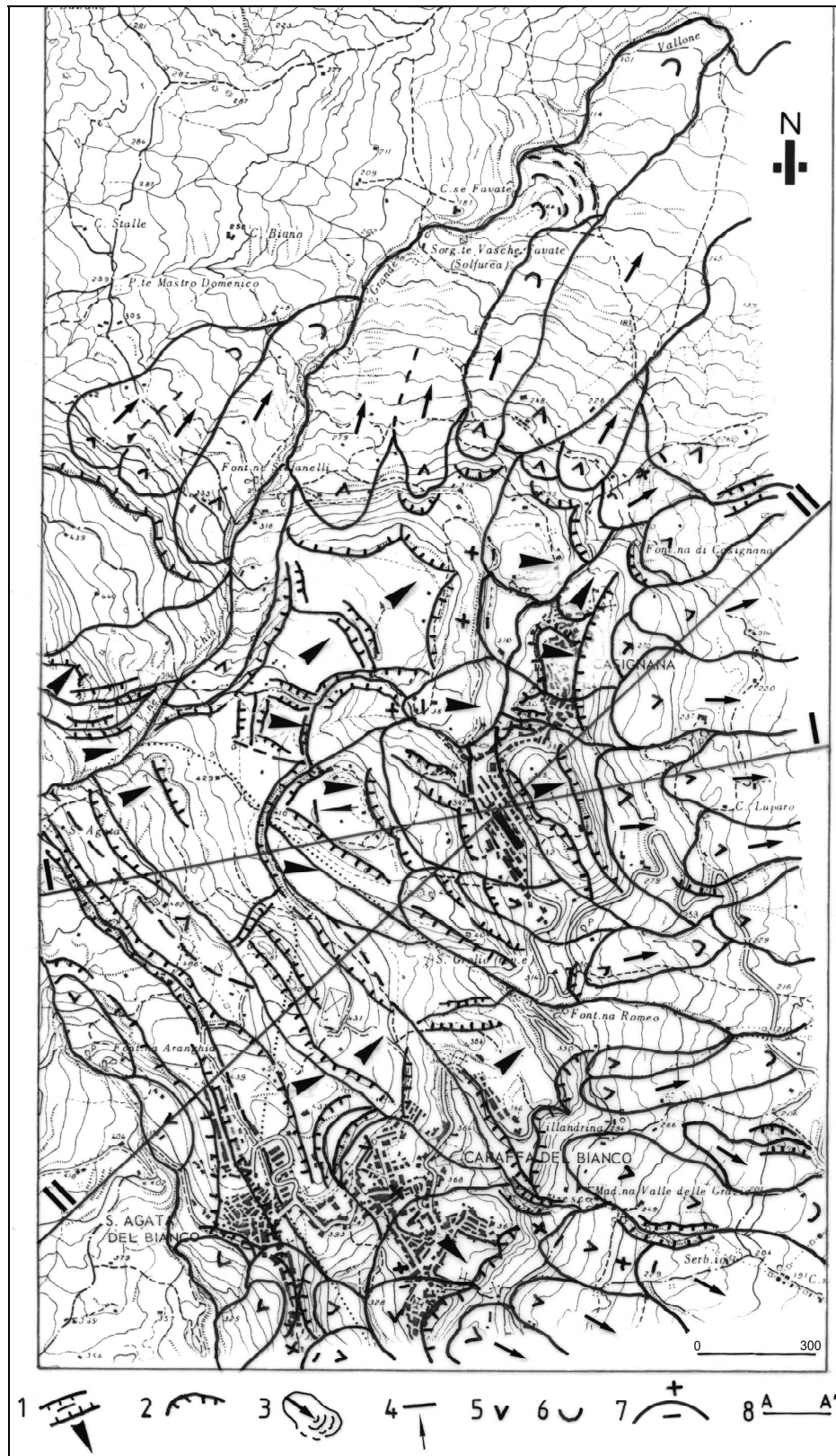
Fig. 22. Geomorphologic map of the lateral spreadings of Casignana, Sant'Agata del Bianco and Caraffa del Bianco (Aspromonte - Reggio Calabria province). 1. Trench; 2. Crown and scarp of landslide; 3. Landslide body limit and direction of movement; 4. Tilting; 5. Slump and slide; 6. Flow; 7. DSGSD rupture; 8. Line of geological section.
